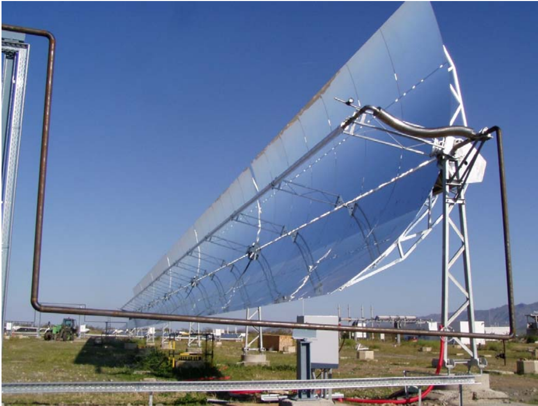
Figure 3: Prototype Albiasa Trough, located in the Plataforma Solar of Almeria (PSA)
